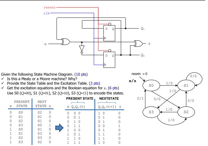
$\begin{array}{l} Q_1(t+1) \leftarrow \overline{x \oplus \left(Q_1(t) + Q_0(t)\right)} \\ Q_0(t+1) \leftarrow \left(Q_1(t) \oplus Q_0(t)\right) + x \overline{Q_0(t)} \end{array}$
